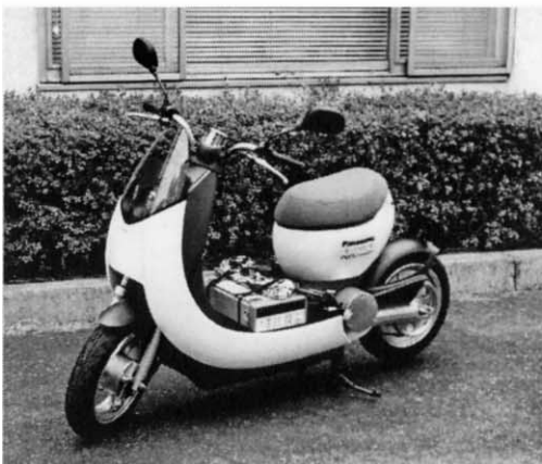
Fig. 12. Some models of middle-size battery systems for near-term practical use: (A) Mini load-leveling device (stationary type); (B) mini electric vehicle (EV) (EV application type); (C) electric scooter-ES-X2 with on-board monitoring device (EV application type).
